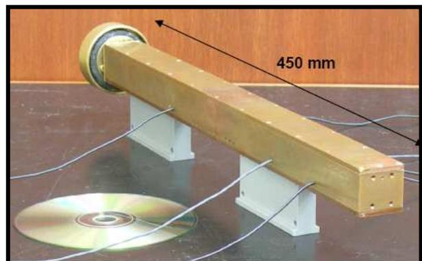
**Figure 1. Gravitec Gravity Gradiometer sensor head. The sensor measures 30x30x450 mm and weighs ~1.3 kg.**
