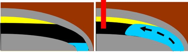
**Figure 3.** An illustration of water ingress along strata. As oil (black) is extracted it is replaced by water (blue) from the permeable source rocks.
