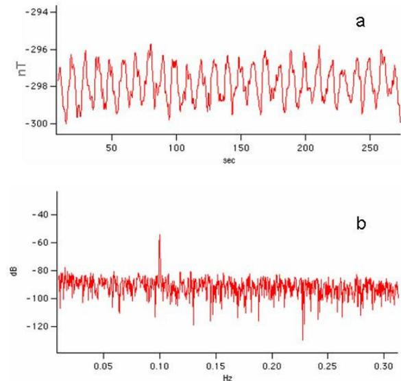
**Figure 2.** Time domain (a) and spectral data (b) recorded from the Magnetic Gradiometer. A magnetic gradient signal of 1.6 nT/m peak at 0.1 Hz is used to determine the sensitivity of the sensor. The noise floor is about 50 pT/m below 0.1 Hz with the cut-off frequency determined by 1 sec integration time. The gradiometer was stationary in an unshielded environment. The raw data has not been improved by removing the DC component in the frequency domain.
