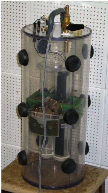
**Figure 1.** A Magnetic Gradiometer sensor mounted inside a 3-stage passive isolator. The sensor itself is 300 mm × 30 mm × 30 mm and weights 200 g. It operates at room temperature in either atmospheric pressure or vacuum. The suspension is employed to provide 3-stage isolation of the sensor from aircraft acoustic and vibration noise.
