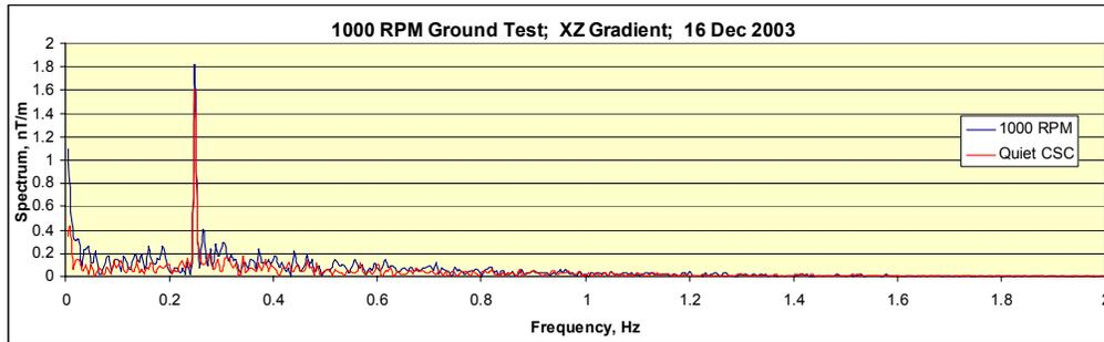
Figure 3: Spectrum for the MG sensor while aircraft engines are running at 1000 RPM. The spectrum is calibrated in nT/m and shows a noise floor of 0.2 nT/m with engines running. The 1.6 nT/m peak calibration signal is clearly visible at 0.25 Hz.
