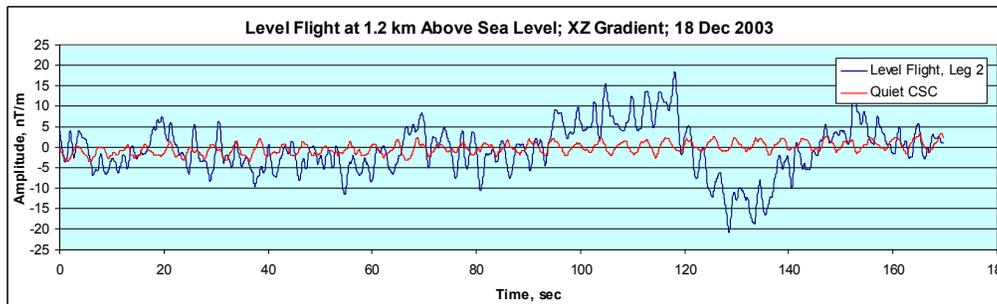
Figure 4: Uncompensated time domain recording for high altitude level flight. Various features on this plot (*i.e.* the gentle increase from 100 s–120 s, the fall from 120 s–130 s, and the rise from 130 s–140 s) correlate with maneuvers of the aircraft in flight, indicating that heading error variation is the cause of these excursions. The GPS altitude is 1200 m and the heading is 167°.
